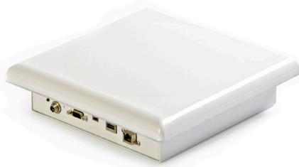
Astra-EX is an easy to install, unobtrusive, integrated 2-port reader/antenna designed for office and commercial environments. Driven by ThingMagics powerful Mercury6e (M6e) UHF RFID Module, Astra-EX's Power-over-Ethernet (PoE) and Wi-Fi options allow for flexible, low cost, single cable installations. Astra-EX blends in well with corporate IT infrastructures and office layouts, and offers full support for ThingMagic's enterprise-class MercuryAPI software
