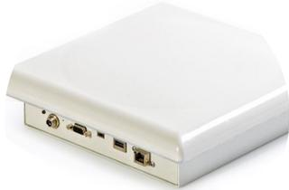
Onboard processing is typically associated with mobile computing RFID readers, but is also available on many fixed readers. A reader with a processor can run applications on the reader instead of running them on a computer. This reduces the need for a host computer in networked applications. Readers with onboard processing typically
