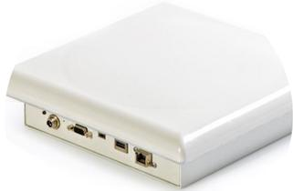
When choosing a reader for an application, the user should always check the amount of available antenna ports. Typically, readers are available with two-ports, four-ports, and eight-ports (without any additional devices, such as **multiplexers**). Antenna hubs, or multiplexers, are available that can connect up to 32 antennas to a single reader. When
