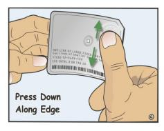
Stick the tag to the glass by rubbing your thumb up and down in a zigzag motion across entire tag surface. Be sure to rub over the tag's chip to remove as much air as possible.
