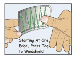
Push out trapped air by rubbing on tag as shown in Step 4, Apply.
