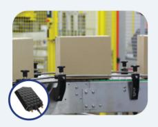
The HID Acura AcuPad-50 and AcuPad-50 MUX are compact and efficient UHF RFID readers designed to deliver high performance across a wide range of industries. Both models come with two SMA outputs for external antennas, providing flexibility in usage and enhancing their adaptability to various operational environments. The readers are powered via USB, combining the convenience of simple connectivity with reliable performance, making them suitable for a diverse set of applications.
