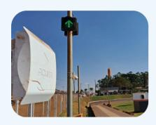
The HID Acura EDGE-30R+ AutoID is a high-performance UHF RFID reader designed for tag reading applications, primarily targeting vehicle access control.
