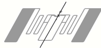
Angular Sensitivity Inlay is rotated in the x, y, plane about the z axis
