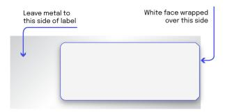
Smallest recommended bending diameter of the **Beontag ESD On Metal Label** is 100mm. For optimal performance please bend the label in the orientation shown below.
