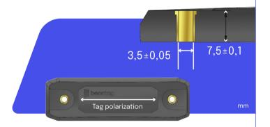
metal surface and tag. DIN 7985 M3 screws can be used as a reference.
