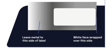
Smallest recommended bending diameter of the Beontag Steelwave Flex is 50mm. For optimal read range please bend the label in the orientation shown below. Note that with smaller assets it is recommended to bend the label to other direction for optimal adhesion.
