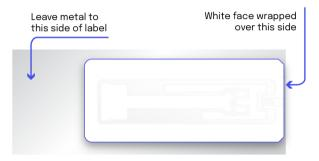
Minimum bending diameter of the **Beontag Silverline Classic II** is 100mm. For optimal performance please bend the label in the orientation shown below.
