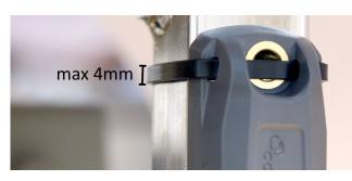
Polarization of Confidex Survivor<sup>™</sup> is according to its longest dimension. This should be taken into account when using linearly polarized reader antennas.
