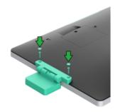
Install the 2 flat head screws included with the kit and cover the screws with the adhesive mylar covers if desired.
