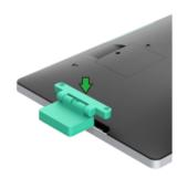
Gently insert the RFID Reader into the peripheral bay taking care to ensure the connector mates properly.
