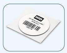
HID IQ On-Metal Labels are small, thin self-adhesive NFC or RAIN® UHF tags for on-metal use. These white PET labels may be encoded and printed in standard label printers to apply logos, bar-codes, QR codes or text (except IQ OM LR®). Their flexible special shielding allows application on flat or curved metallic objects like liquid containers, laptops, pipes or machinery.
