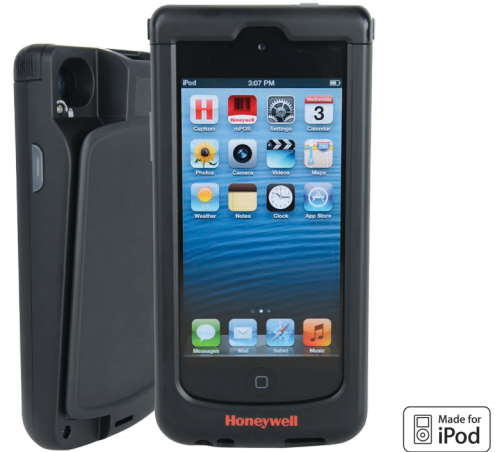
The Captuvo SL22 enterprise sled transforms the Apple iPod touch into an enterprise-ready device that can scan barcodes and check out customers from anywhere in the store.
