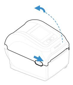
Slide the printer front door up and remove it from the printer.
