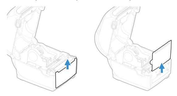
Slide the cutter module down to the front of the printer until it locks in place.
