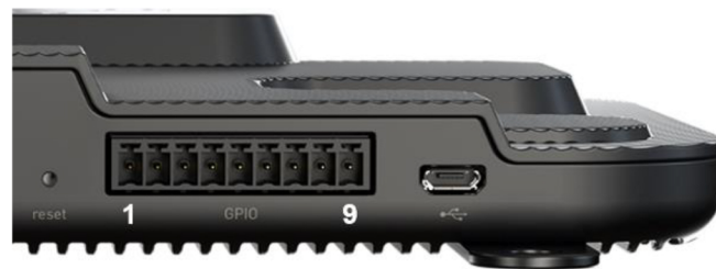
Figure 8: Impinj R700 Series GPIO Pin Locations
