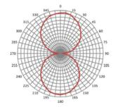
Angular Sensitivity (Relative Read Range vs. Orientation)
