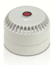
Model LP4 low profile, electronic piezo sounder is a compact multi-tone sounder ideal for OEM and general alarm applications. The low voltage LP4 provides the user with the choice of 32 different tones, selectable during installation. Each electrical connection has two terminals for looping in and out, eliminating the need for a separate terminal block, making installation easier. A second tone is available if a third wire is installed and connected to the second tone terminals.
