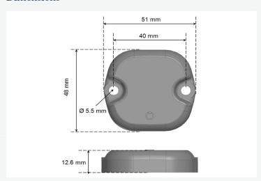
Measurements shown in mm
