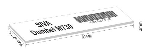
SIVA's RAIN(UHF) RFID foam transponders are ready to apply foam backed race timing tags on marathon bibs and are designed to ensure athletes receive the most accurate measurement of their timings while they race.
