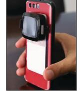
The SLS M-101 Keyboard Wedge version connects to any operating System as a wireless keyboard and outputs RFID data directly to a text file, spreadsheet, web form, etc. without the need for application development.
