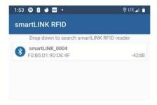
The "0004" corresponds to the last 4 digits of the serial number of the smartLINK (visible on the back of the device).
