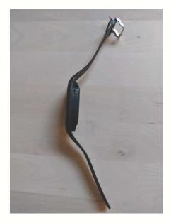
The smartLINK can be charged via micro USB. Connect directly to the port on its side (shown in photo).
