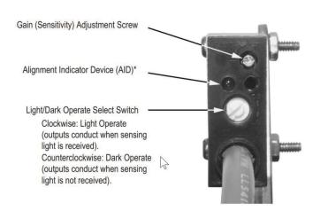
The default setting on the photo eye sensor is dark operate which means it will send a falling (high-to-low) transition output if it does not sense a reflected beam (the beam is 'broken').
