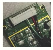
8. Attaching the USB "Y" Cable to the end of the USB cable to the board is optional. When attached, the black USB end is connected to the host PC and the red end may optionally be connected to a second USB port (or a USB charging plug) to provide extra DC power should a single DC power of the port on the PC host be insufficient to power the module when the module is transmitting at its highest RF power levels. The default settings do not require use of the USB "Y" cable.
