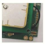
5. Use the nylon hardware to mount the antenna to the board in 4 locations, as shown below.
