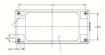
Alternatively, rubber feet can be mounted over the inserts in the detents provided.
