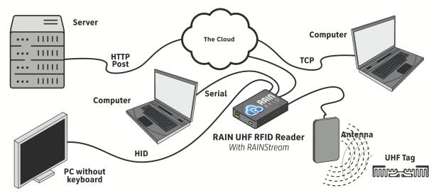
RAINStream allows direct transfer of tag data to backend systems via several alternative protocols
