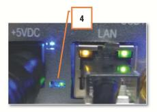
4 - When the green LED to the right of the power connector turns on, the reader has obtained a network address from the network's DHCP server, or negotiated one with your PC. This can take several minutes.
