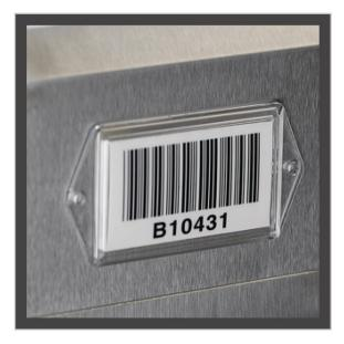
Impact-resistant housing combined with an ultrasonically welded seal protects the subsurface printed label and RFID inlay from harsh environments including harmful UV rays. Affxing methods include mechanical fasteners (standard) and/or adhesive (optional).
