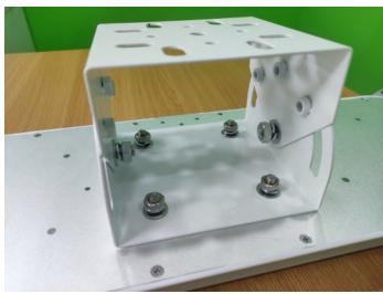
Step 3: Fix the dog tooth fixture on the bracket 2 with M10 nut, flat washer and spring washer
