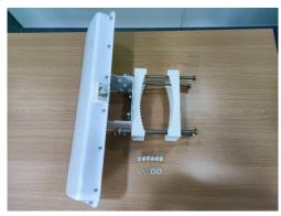
Step 5: Adjust the screws on bracket 1 and bracket 2 to get the right mounting position.
