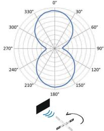
\*Read range drops to 23% of maximum when inlay is perpendicular (90° and 270°) to the reading antenna.
