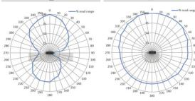
Radiation patterns for the embedded version will vary dependent on the geometry and composition of the asset type.
